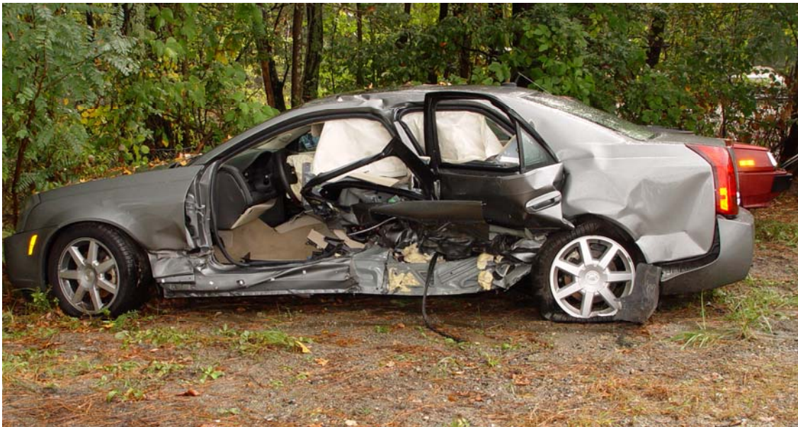
Left side of Cadillac: note damage starts behind front wheel and deepens at "B" Pillar
